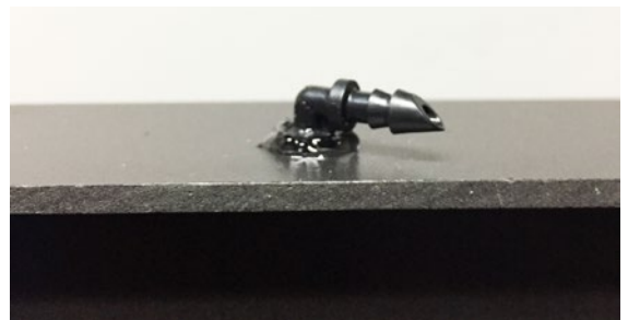
Installing an elbow
